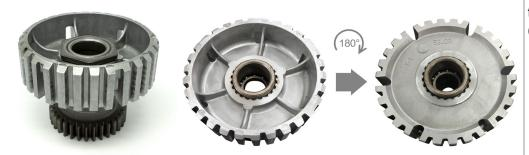
Removed the hub, <u>you need to machine its side (the hollow one) and lowering it of 0,5 mm (see picture below).</u>
