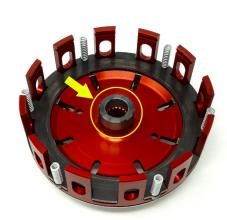
Before coupling the outer bell, <u>remember to put the spacer that was inside the orginal clutch (part not supplied by Jetprime) in the same position</u>, between its internal side and the hub's retaining bolt.
