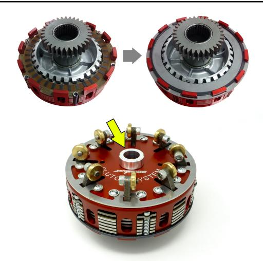
Assemble the complete clutch unit on the engine again, placing our aluminum spacer on the clutch pivot, outside the bell, before tighten the retaining nut with 65 Nm (following Yamaha manual) and lock the new clutch unit. Fill the water and oil engine tanks again.
