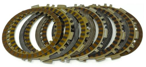
**Please note**: the gauge measurement of the correctly coupled disc pack is approximately 24,5 mm.
