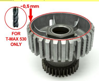
Once the part has been machined, rotate the hub of 180° and couple it with the gear again, then tighten the nut with a torque of 90 Nm.
